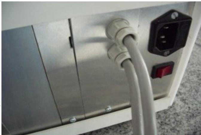
Due to the backplane connector used, each pin can carry maximum 1Ampere (and the voltages are also specified). If more current (or higher voltage) is necessary, or when special cables have to be used, the connections have to be made via back panel.
