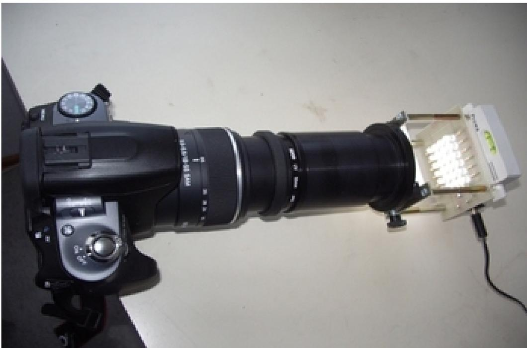
I improved it to have a customized LED light (containing 6 times 4 single LEDs).
